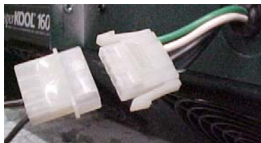
White bypass plug connections are used on most units manufactured before 2003.
